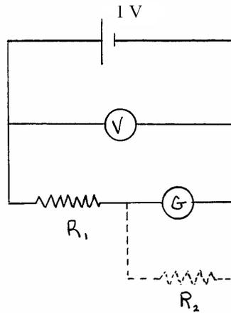
Now back to the circuit without  $R_2$  present; since the galvanometer is fully deflected, Ohm's law permits you to compute the current for full-scale deflection. (Read potential from the voltmeter and the resistance is the sum of  $R_1$  and  $R_g$ .) Call this full-scale current  $I_g$ .
