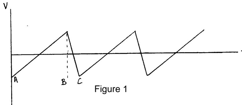
This is a plot of voltage versus time; the lowest voltage (point A in the figure) corresponds to the beam at the left side of the face of the CRT, and the highest voltage (point B) corresponds to the right side. The voltage at the midpoint is half the maximum. The voltage decreases rapidly from B to C to repeat the trace. The sweep rate is adjustable.
